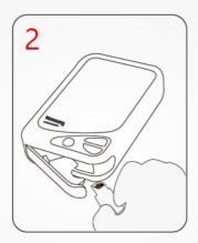
2. Place the filled cuvette in the cuvette holder and push it back.
